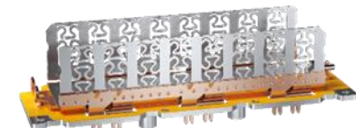
Inverter assembly with insulation foils
